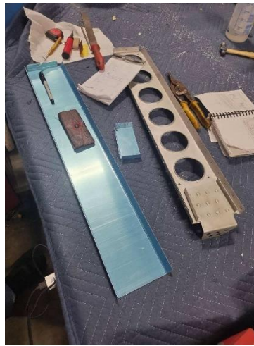
Above: I will finish my time at Missionary Maintenance Service (MMS) Aviation in Ohio on February 24 th . For my last few weeks at MMS, I assisted with installing the interior in a King Air aircraft and helped get it ready to return to service. I had a sheet metal project where I fabricated a stringer for a Cessna 207 heading to Gabon, Africa. A stringer is like a floor joist of the aircraft. In addition, I manufactured a bracket for an airplane component that helps the plane turn, and I helped rivet the floor back on a Cessna 206 from Mexico.
